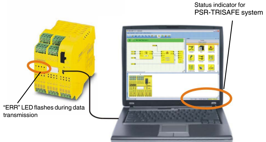
Figure 10-4 USB connection between PC and safety module
