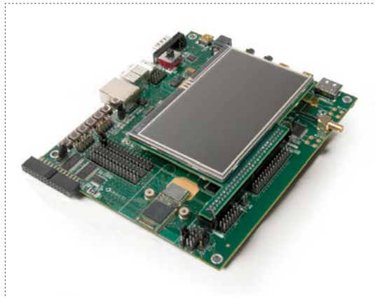
ZOOM DM3730 TORPEDO DEVELOPMENT KIT WITH DM3730 TORPEDO + WIRELESS SOM & 4.3" WQVGA LCD INCLUDED
