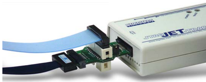
FIGURE 38 The JTAG-ETM splitter board attached to the JTAGjet-Trace emulator. Connected to it are a 20-pin ARM JTAG cable and an ETM Mictor cable (lower). A receptacle for an additional 14-pin TMS320 DSP JTAG cable is located at the bottom of the board.
