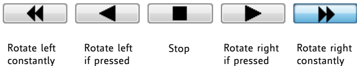
Figure 8.4 Jog tab keys for moving a motor
