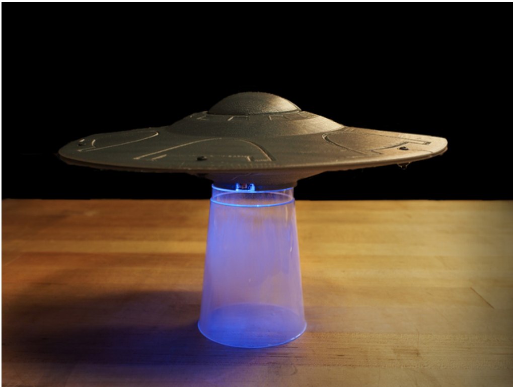
UFO Flying Saucer by John Park uses the accelerometer tilt to control lights and sounds on a fun flying saucer.
