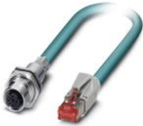
Flush-type connector M12, 4-pos., D-coded, for rear mounting, with Ethernet cable AWG 26 stranded (7-wire) and RJ45 connector, length: 0.3 m
